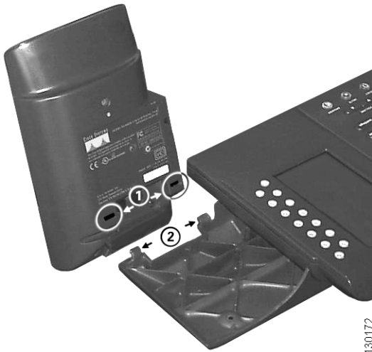
Figure 4 Connecting the Expansion Module to the Support Bar
